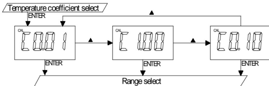
Pressing **[UP]** key or **[DOWN]** key in this screen will cycle the display from C1.00, C0.10 to C0.01 basic cell constant above.
