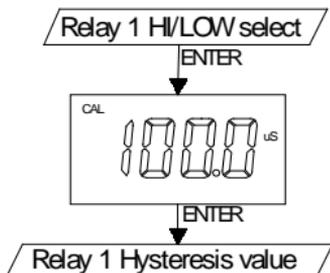
Pressing **[UP]** key or **[DOWN]** key in this screen to adjust the value, press **[ENTER]** key to save, and enter the next setting screen.
