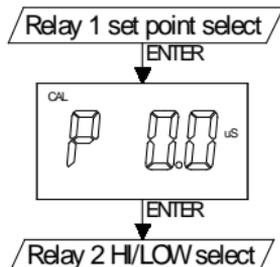
Pressing **[UP]** key or **[DOWN]** key in this screen to adjust the value, press **[ENTER]** key to save, and enter the next setting screen.
