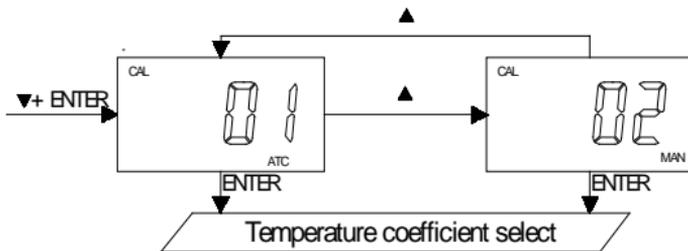
Pressing **[UP]** key or **[DOWN]** key in this screen will cycle the display between 01 (Thermistor: 10k ohm), 02 (Manual) modes above.
